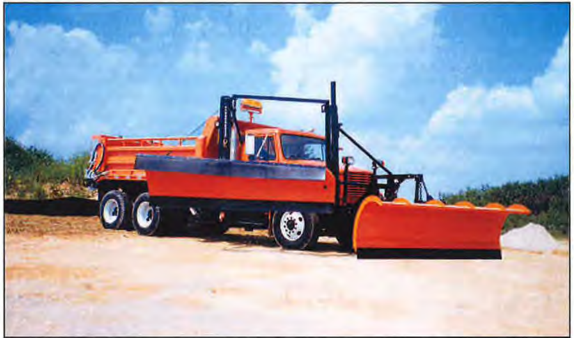
Shown in benching position with optional rubber snow deflector and a Monroe Reversible Snowplow.
