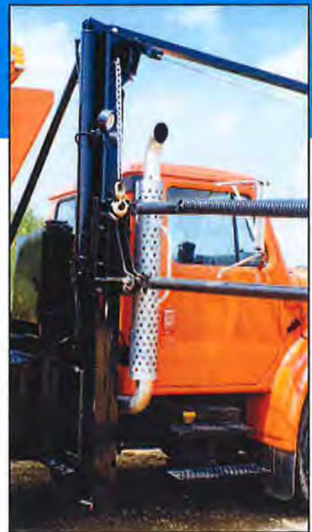
Rear wing post with 3-position adjustable pusharms
